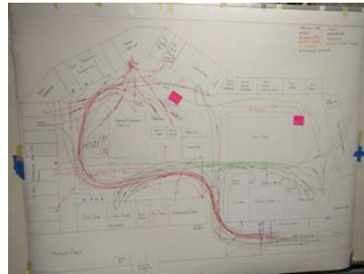
Representatives from each trade shop mapped a spaghetti diagram of their dispatch routes, indicating the bottleneck at the entrance/exit
